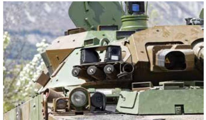
The PeriSight® is a patented **network of imaging sensor modules** offering multiple viewing channels - low light color and thermal. The system provides **night and day 360° surveillance** in short and long range (in zoom version) to enhance **Land Situational Awareness (LSA)** and **Driver Vision Enhancement (DVE)** for driving and manoeuvres.
