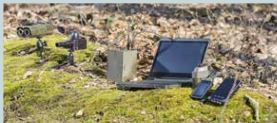
Wireless mesh networked Unattended Ground Sensor (UGS) platform
