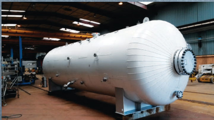
85m 3 - 40 T, working pressure 35 bar
