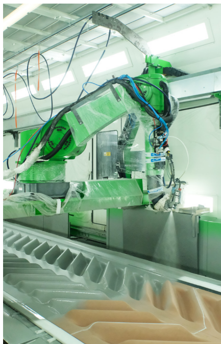
Robotic polyurethane spraying.
