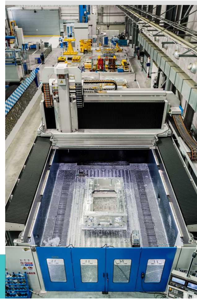
Double gantry milling machine (X 30000, Y 9000, Z 1250 mm, maximum load: 5 tons / sqm).
