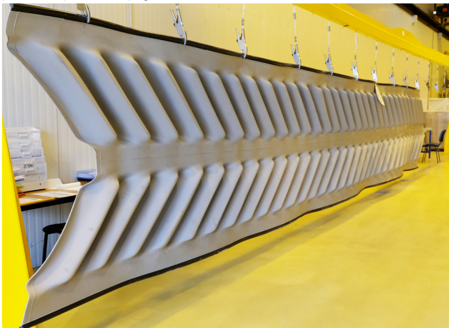
Part of the membrane sealing Chernobyl Safe Confinement.
