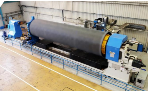
Horizontal lathe (L 15000 mm, maximum load 40 tons).
