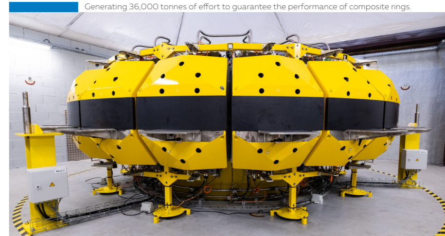
Generating 36,000 tonnes of effort to guarantee the performance of composite rings.
