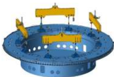
Figure 1: Lifting beam to install the cryostat base section (1,250 metric tons)
