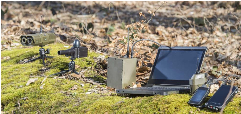
Unattended Ground Sensor (UGS) networks ©T.Leaud - Exensor
