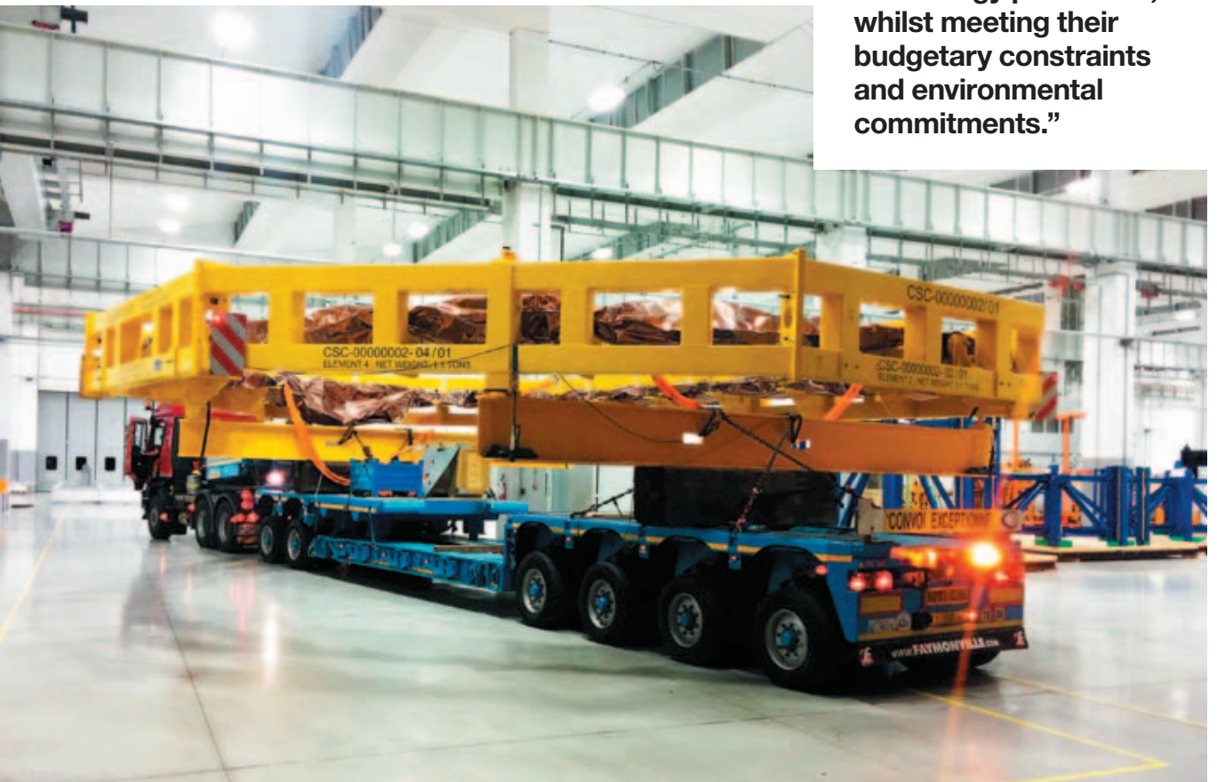
Top. A mobile production line for solar panel casings intended for a concentrated solar power plant. Bottom. A radial plate for the ITER reactor leaving CNIM's industrial site.
