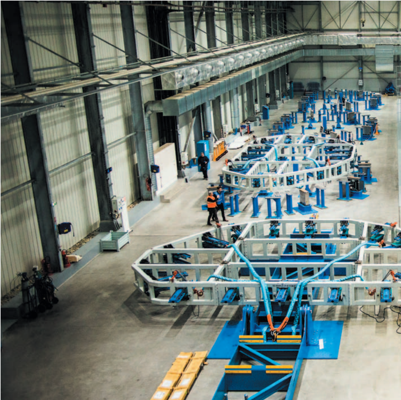
Factory at CNIM's industrial site at La Seyne-sur-Mer where the radial plates for the ITER reactor are manufactured.
