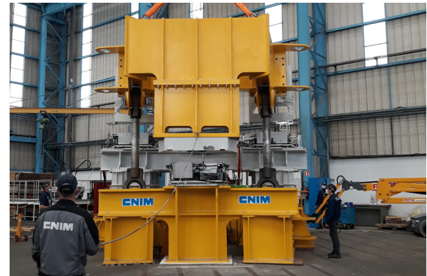
Testing one of the tools for mounting components for the ITER fusion reactor.
