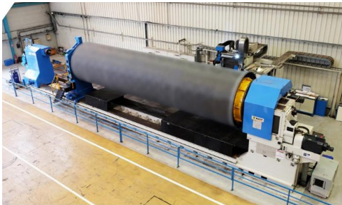
Horizontal lathe (L 15000 mm, maximum load 40 tons).
