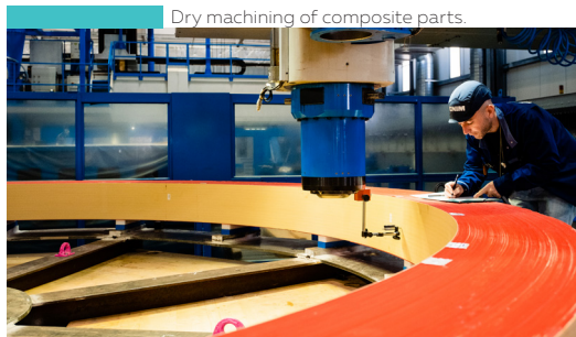
Dry machining of composite parts.
