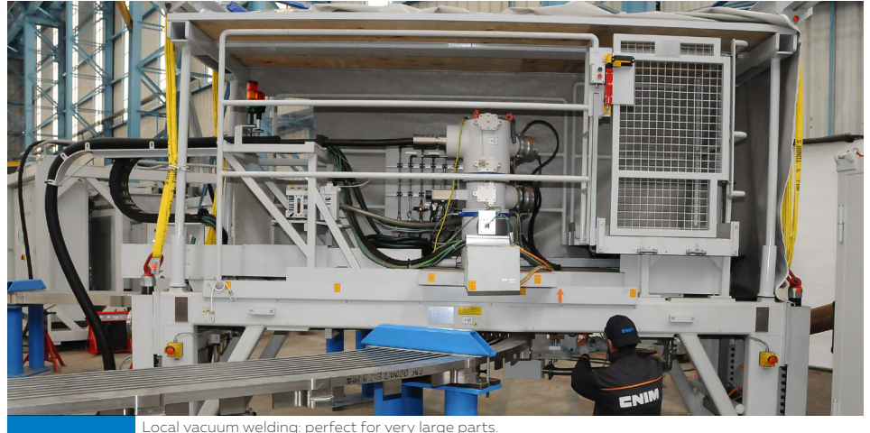
Local vacuum welding: perfect for very large parts.
