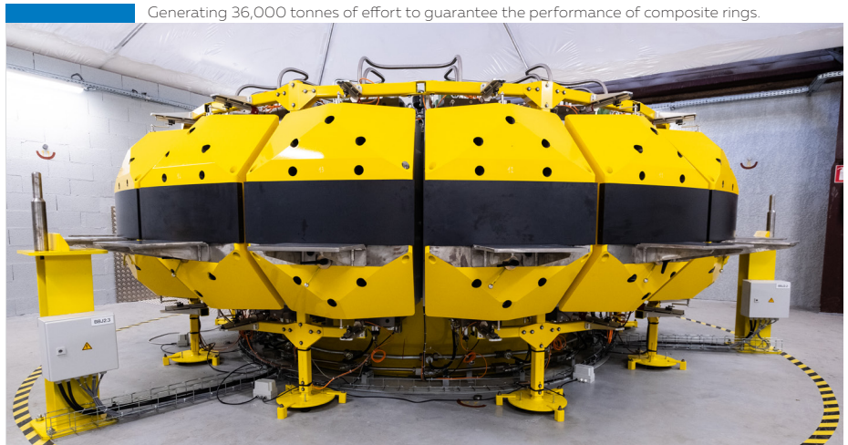
Testing one of the tools for mounting components for the ITER fusion reactor.
