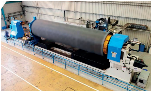
Horizontal lathe (L 15000 mm, maximum load 40 tons).
